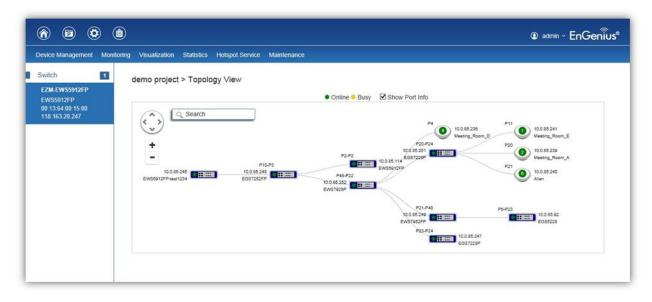
If you have an EWS Switch deployed in your network, you will be able to see a visual view of the topology of all supported devices in the network. The Topology View feature will automatically maps your network deployment and displays the device relationships across your network infrastructure. An essential feature for troubleshooting network issues that would otherwise require manual mapping, overlay monitoring software, or manually keeping track of MAC address tables.
